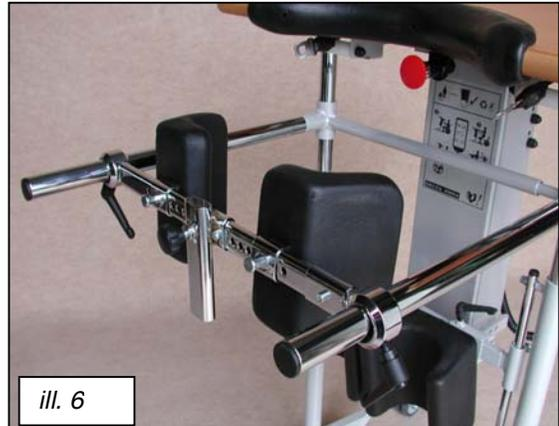
To adjust the height of the hip support rails undo the clamping handles on the top chromed section of the vertical tubes. There is no additional height adjustment control in the hip support rails so caution must be taken to support the rails when adjusting their height. Hold the rails as close to the handles as possible to ensure the rail moves smoothly. Raise or lower the rails to the desired height and tighten the clamping handles. Ensure the rails are firmly positioned before using the Delta.
